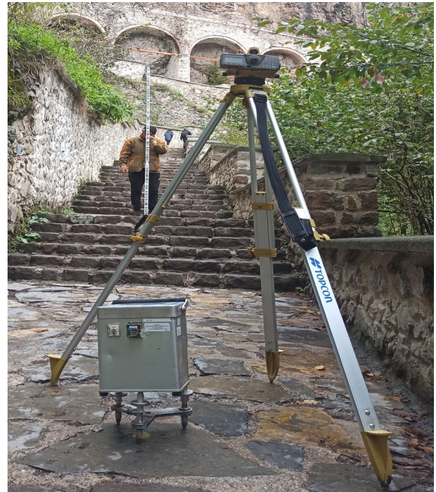
Fig. 2 Simultaneous gravity and leveling measurements
