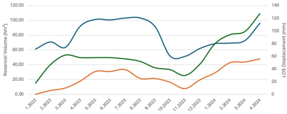
Fig. 9 The displacement rates at monitoring point in dam crest PS are presented with descending LOS results in orange, ascending LOS in green, and reservoir water volume measurements in blue
