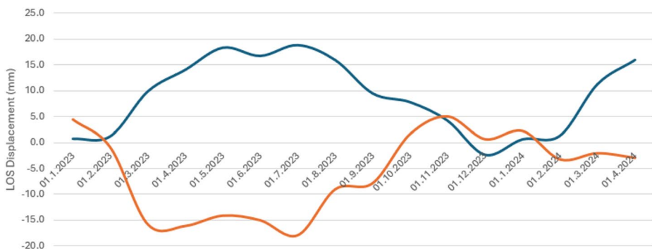
Fig. 3 The displacement rates at monitoring point P3 in dam crest, as observed through PS-InSAR analysis, are presented with descending LOS results in orange and ascending LOS results in blue
