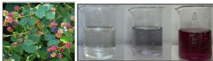
Fig. 1 Visual observation of AuNP formation using the aqueous fruit extract of Rubus caesius L.: (a) fresh fruits used for extract preparation; (b) initial reaction mixture containing \text{HAuCl}_4 \cdot 0.3 \text{H}_2\text{O} solution and the aqueous fruit extract before microwave irradiation; (c, d) reaction mixture after microwave treatment, showing the development of a distinct purple–pink color that visually suggests the formation of gold nanoparticles (AuNPs)
