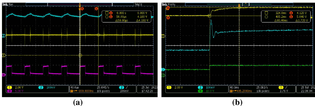
Fig 14. Open-loop system response at 20 kHz switching frequency a) 0.3 duty cycle, b) duty cycle change from 0.3 to 0.5.
